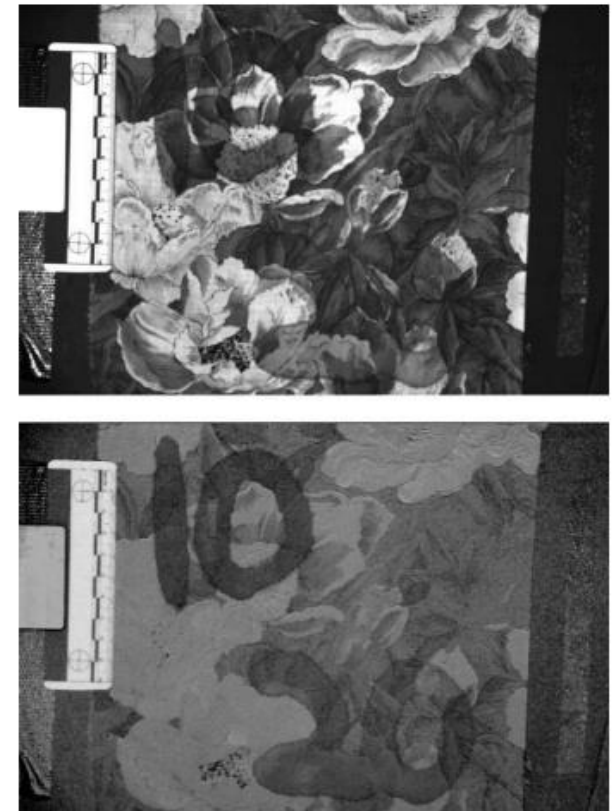
Figure 3: Images of 10-fold and 20-fold diluted blood on a floral substrate. Top image was taken at 415 nm. Lower image was obtained by performing background correction according to equation 2. Both images have been adjusted for optimal brightness and contrast.
